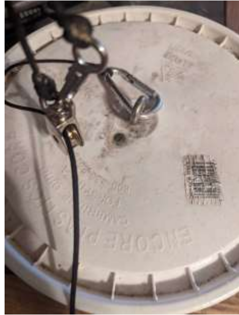
Scion (lid) with rope attached to eye screw and pulley
