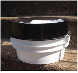
Upper portion of bucket flipped over to wedge paper towel filter in place
