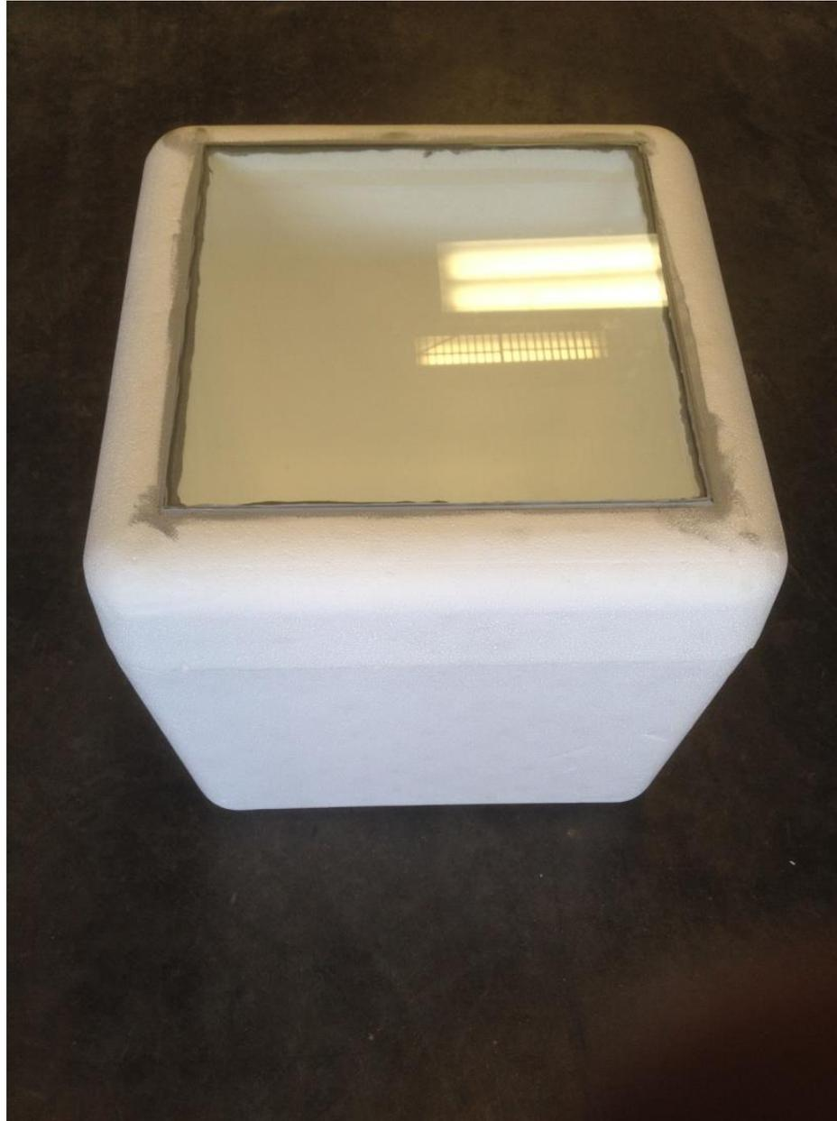
***With a razor blade, clean up excess silicone sealer & chamfer inner edge***
